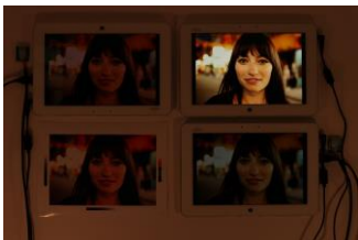
Figure 1: "Calm display" mode used in this probe, under different lighting conditions. In each photo, calm display at top left, printed paper at bottom left and normal display at top right. [8]
