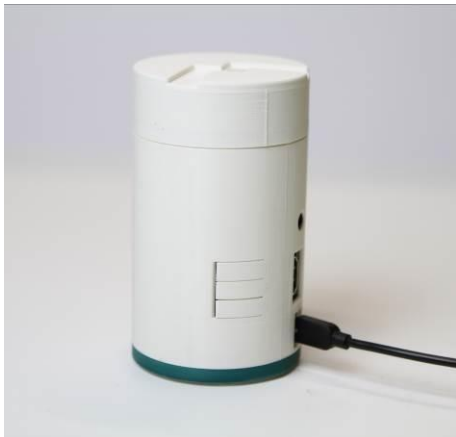
Figure 1: The meSchHub allows the rapid interweaving of arbitrary devices and communication technologies. Tapping a NFC enabled smartphone on the meSchHub will instantly connect it to its embedded WiFi access point and give access to its web based GUI
